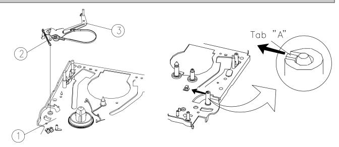
Fig.3-15 TENSION BAND ASSY REMOVAL (I)
